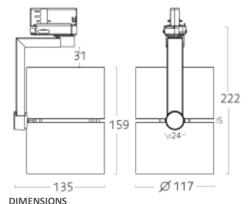
Length, mm 117 Width, mm 136 Height, mm 256 Weight, kg 1.2
