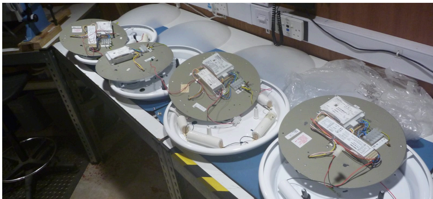
Remanufacture in progress — the original housings and diffusers retained, new gear trays built to the approved specification of 18 May 2023.
