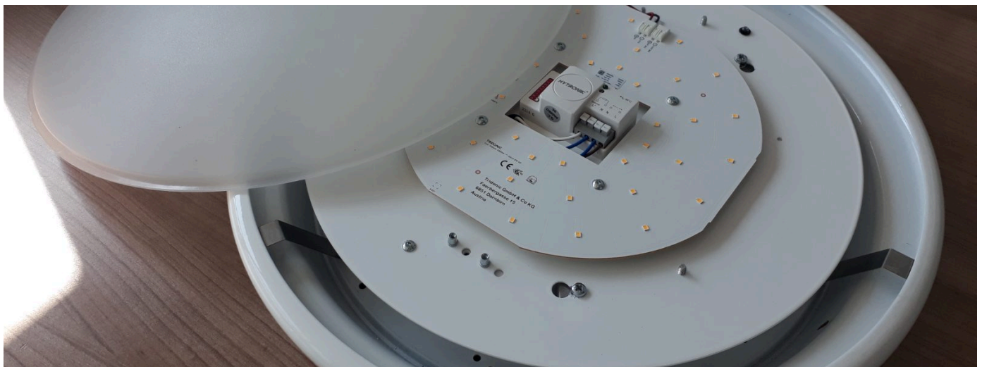
A remanufactured bulkhead opened — new LED module and microwave sensor inside the retained housing.
